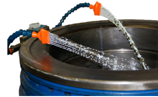
Chris-Marine honing head equipped with vibration dampers for optimum performance.
