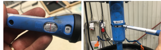
Adjusting torque wrench (left) and setting stone pressure (right) with HON S and HON A.
